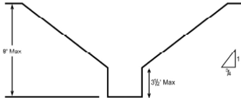
All excavations more than 8 feet but not more than 12 feet in depth with unsupported vertically sided lower portions must have a maximum allowable slope of 1:1 and a maximum vertical side of 3 1/2 feet.
